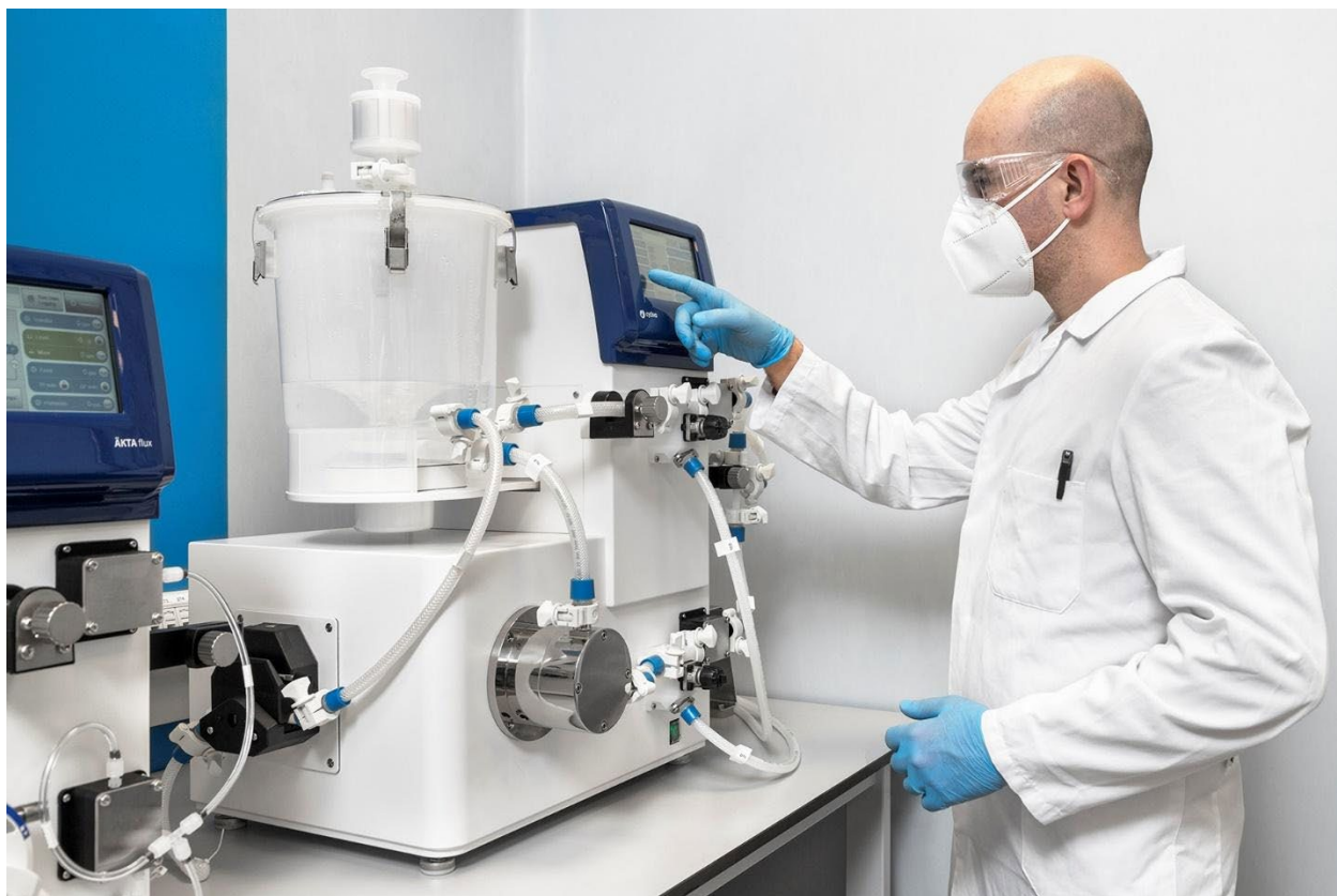
CordenPharma Caponago (IT) LNP R&D Laboratory: TFF equipment for diafiltration and concentration of Lipid Nanoparticle formulations.
